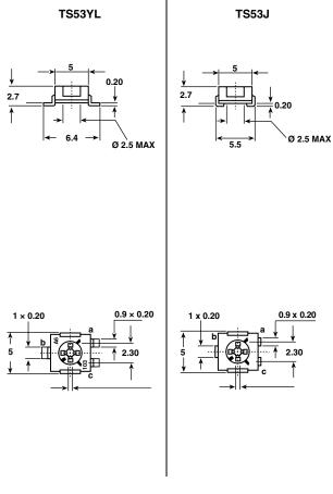
cruciform screwdriver slot ø 2.5, width 0.5 deep: 0.55 max deep (center): 0.7
